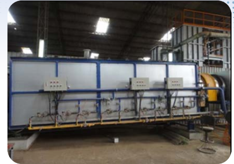
Second Section 0.95m(dia.)x12.0m(L)
