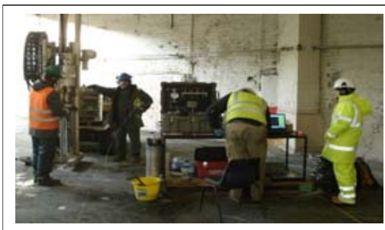
FIGURE 2. Modified Waterloo Profiler Investigation, showing Geoprobe™ and field sampling equipment.
