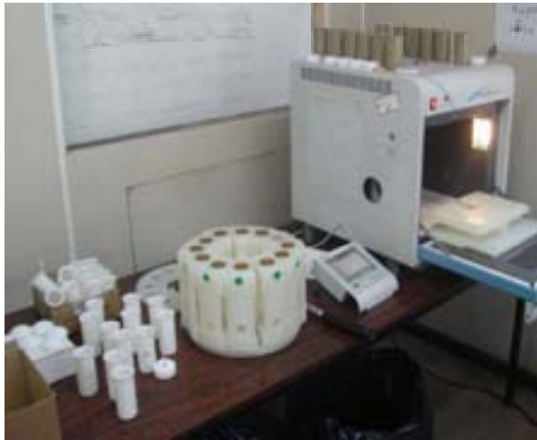
On-site laboratory analysis of pore water concentrations using Microwave Assisted Extraction
